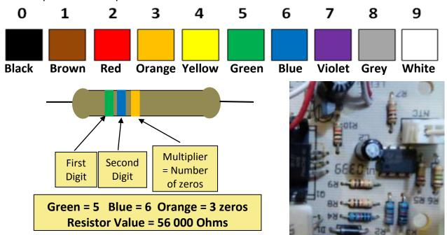
1. Work out the values of the resistors below.
